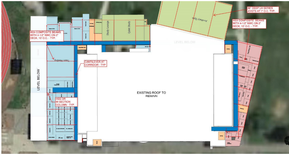
Structural Diagram: Level 3 Framing Concept
