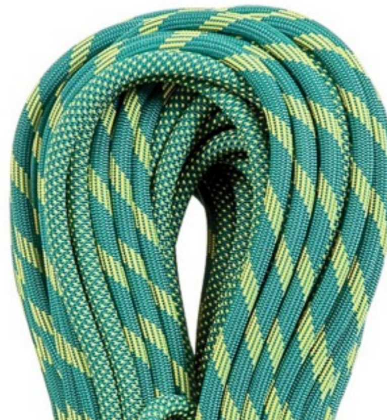
Climbing rope is composed of woven Nylon (a polyamide, condensation polymer). The elasticity of the rope is intrinsically linked to the molecular structure of the polymer backbone.
