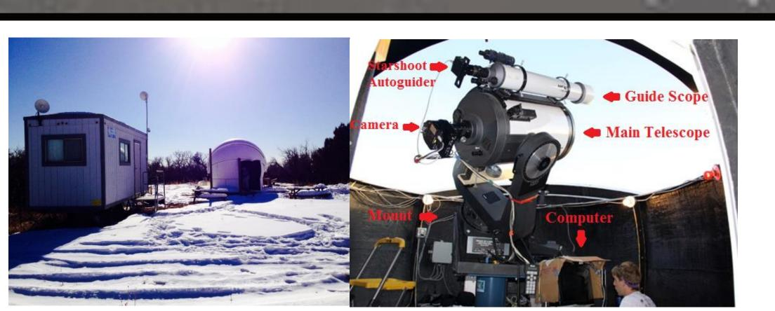
The Fort Lewis College observatory (left), and the 16" telescope with its CCD camera, mount, and guide scope with camera (right). This experiment will help determine if the equipment at the Fort Lewis College Observatory is sensitive and precise enough to reliably detect the change in brightness of a star due to a transiting known exoplanet.
